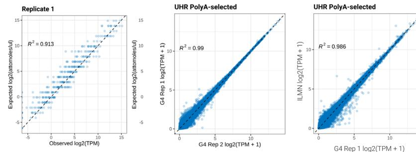
PolyA-selected RNA-Seq libraries were prepared from UHR RNA (Thermo Fisher Scientific) with an ERCC spike-in, sequenced via 2x100bp reads on G4 and Illumina NextSeq 2000 platforms, then downsampled to 25M read pairs for analysis via STAR<sup>1</sup>.
